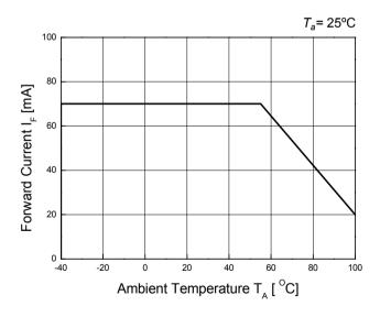
**Ambient Temperature vs. Forward Current**
